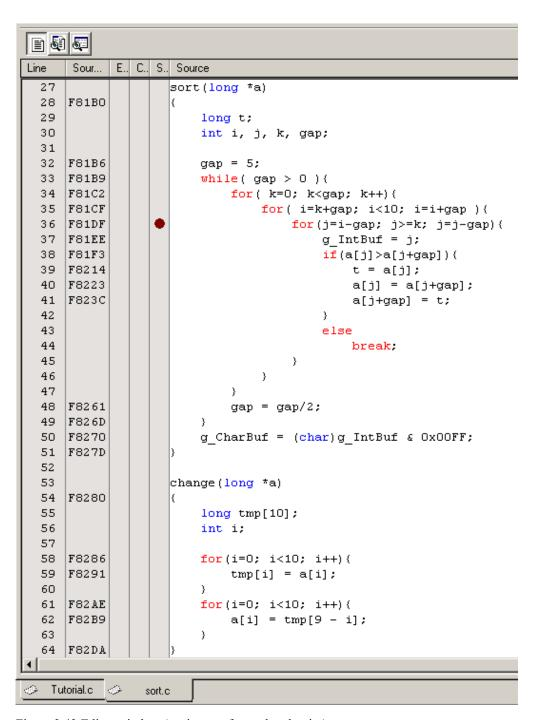
Figure 3.43 Editor window (setting a software breakpoint)
